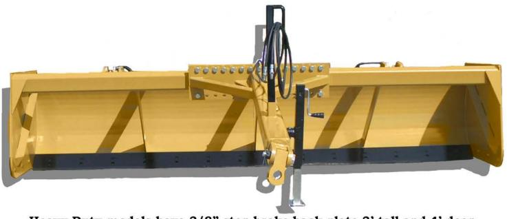
Heavy Duty models have 3/8" step broke back plate 3' tall and 4' deep. Blades are 3/4 x 8 reversible.
