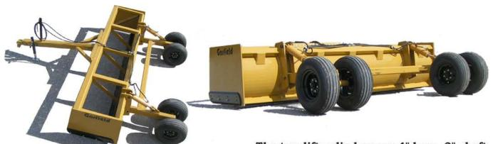
Sides are reinforced 5/8" plates. All models have 22" Ground Clearance. The two lift cylinders are 4" bore, 2" shaft and 12" stroke. The tires are 11L X 15.
